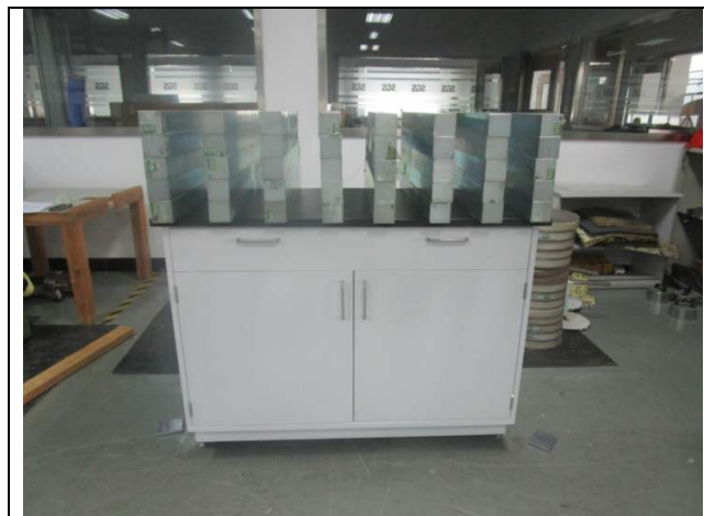
Cabinet Load Test
