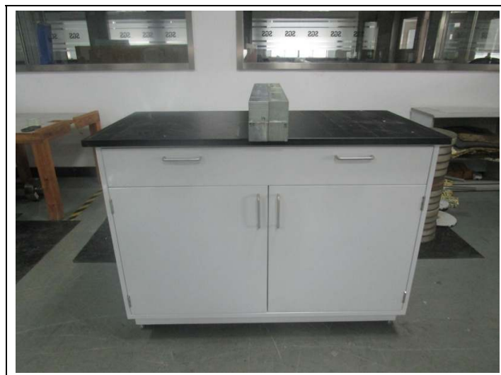
Concentrated Load Test
